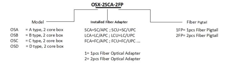
For example: OSA-2SCA-2FP, A type 2 core box, installed 2pcs SC/APC Adapter and Pigtail
